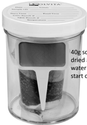
40g soil pre-dried at 45C and water added at start of test
